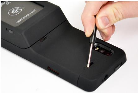
**12** Slide the locking tab over to the right to release the top cover from the case.
