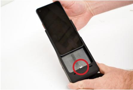
**9** Slide the device into the other side of the case. Ensure that the power port on the device will align with the connector in the case.
