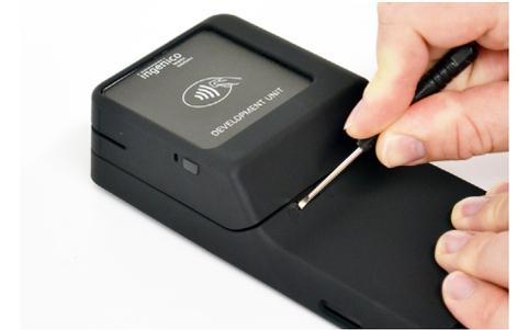
**15** Slide the locking tab over to release the card reader cover from the case.
