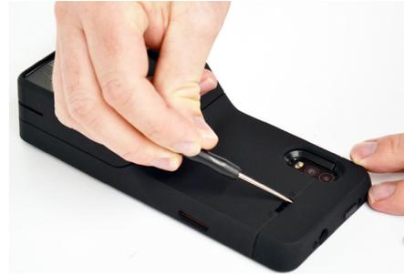
**11** Slide the locking tab over to the left to secure the top cover to the case.
