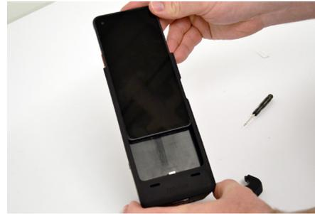
**14** Slide the device out of the case.
