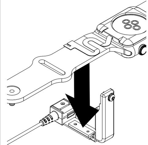
**14d** Plug the tray flex sensor connector into the port on the inside of the band clamp.
