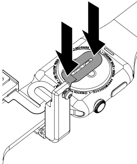
**16** Close the band clamp over the watch band and flex sensor.
