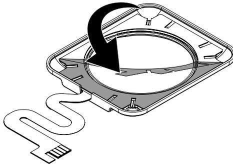
**14b** Place the tray flex sensor onto the bottom of the wearable. Make sure that the connector is facing towards the back band. Apply pressure for at least 10 seconds.
