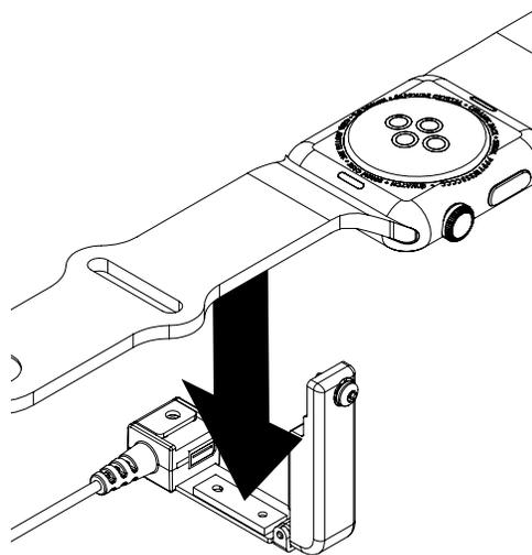
**15b** Plug the universal flex sensor into the port on the inside of the band clamp over the wearable.
