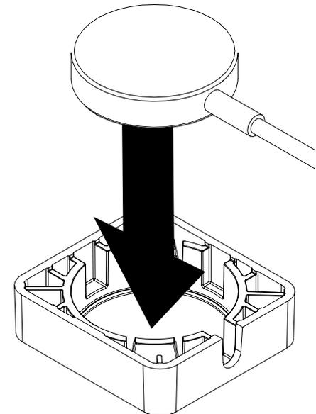
**2g** Route the OEM charger cable into the cable guide.
