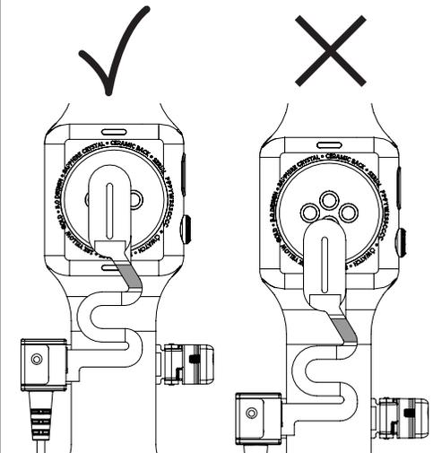
**15d** Peel the liner from the adhesive portion of the flex sensor.
