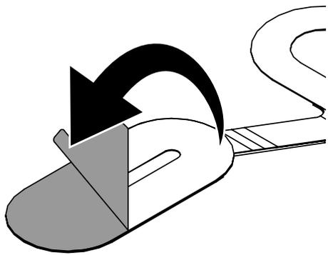
**15e** Press the flex adhesive against the bottom of the wearable for at least 10 seconds. Ensure that all of the oval is adhered to the wearable and that no gap is visible.
