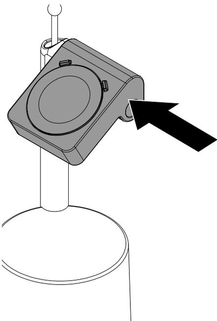
**6e** Secure the custom charger cradle with the screw. Insert the plug into the hole in the side on the cradle.
