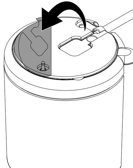
**4 Optional:** Route the power cable through a hole or slot in the fixture.
