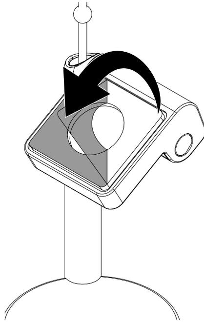
**2i** Place the OEM charger/cradle assembly onto the cradle. Make sure that the adhesive sits in the depression and press the trim piece, NOT the charger, against the cradle for at least 10 seconds.
