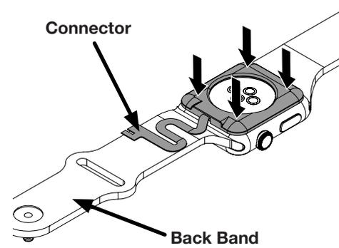
**14c** Place the back band into the open band clamp.
