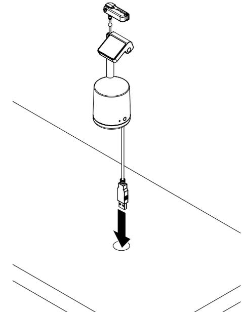
**5** Place the stand in the desired location and apply pressure for at least 10 seconds.
