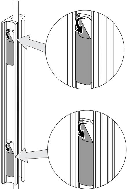
**2l** Align the bottom of the cable guide to the top of the base. Apply pressure for at least 10 seconds.
