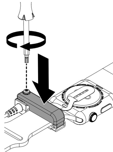
**18** Remove the cable stop clip from the cable.
