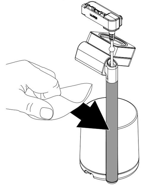
**2k** Peel the clear film from the 2 adhesives from the cable guide.
