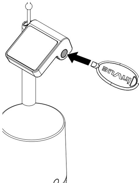
**6b** Remove the plug and screw from the side of the cradle.
