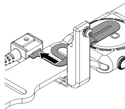
**15c** Adjust the wearable so that the area between the 2 white lines on the flex sensor (the shaded area in the below image) will sit over the "hinge" area (the area where the band connects to the watch body) of the wearable.
