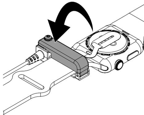
**17** Press down on the band clamp and use a TT8 bit to tighten the screw in the band clamp. Do NOT overtighten.
